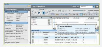
CAD incident, sub-events and recorded media are displayed on the time line, enabling detailed, clear, fully synchronized incident reconstruction.
